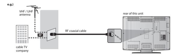
\* Once connections are completed, turn on the unit and begin initial setup. Channel scanning is necessary for the unit to memorize all available channels in your area. (Refer to "Initial Setup" on page 12.)
